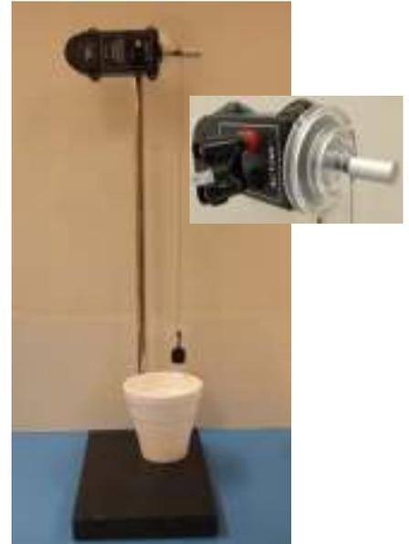
**Figure 2 Experimental Set-up.** The thread is tied to the mass on one end and quadruple knotted at the other. The knotted end is placed in a notch that is in the pulley.
