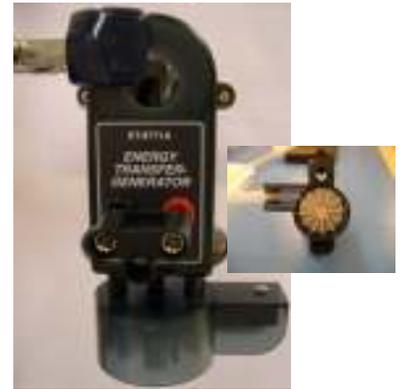
Figure 2 This is ET-generator with the impeller housing and impeller attached. Right, this is what the ET-generator should look like under the housing after step 4.
